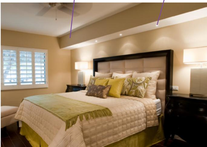
The spots, as in this picture, will be on the bottom of the overhang above each bedside table for a nightlight. Each side will have a switch for their own light and for the LED strip wall wash as above.
